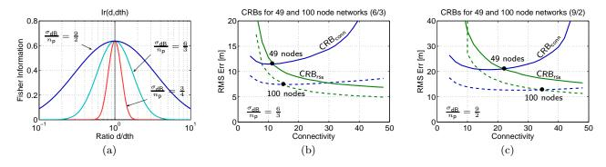
Figure 5: Effect of increasing the number of nodes and the ratio  $\sigma_{\rm dB}/n_{\rm p}$  on the critical connectivity.
