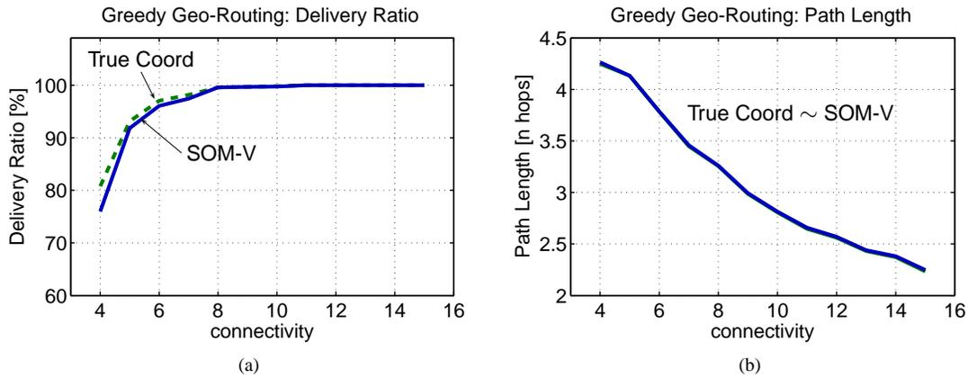
**Figure 3.8:** Average performance of a greedy geo-routing algorithm using the true coordinates and the virtual maps produced by SOM-V: a) Delivery Ratio; b) Path Length. The path length plots (right) are almost completely overlapping for the two cases.
